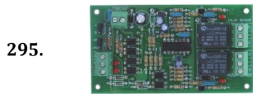
295. COMBINATION CARD / WEFT END + LOGIC CARD PCB A LSL6 1637 33
